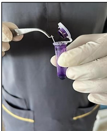
Figure 2: Wire is stained with 1 percent Crystal Violet for 30 minutes
