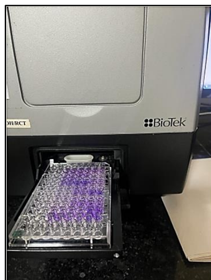
Figure 6: 96 Well Plate is placed into the microplate reader
