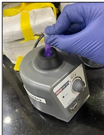
Figure 4: For better solubilisation of dye in Ethanol, wire is vibrated on the vortex.
