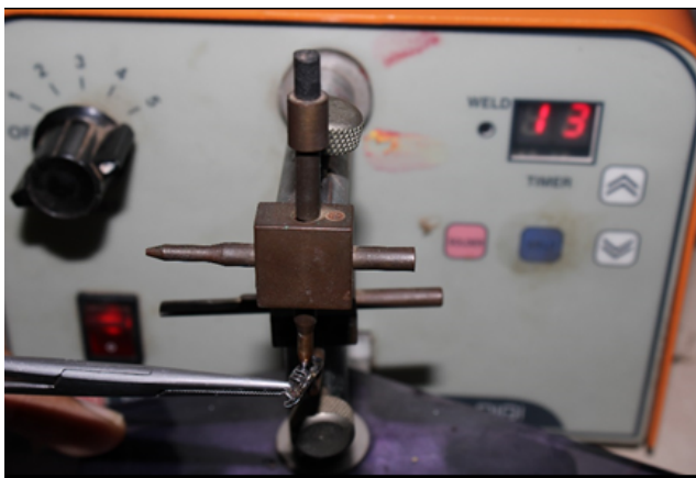
Figure 2: Welding palatal sheath with band material
