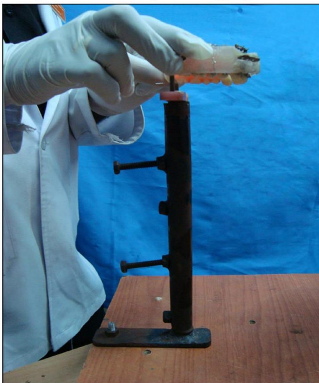
Fig 7. Acrylic rim being fitted to the flat acrylic plate fixed to the top of the copper pedestal
