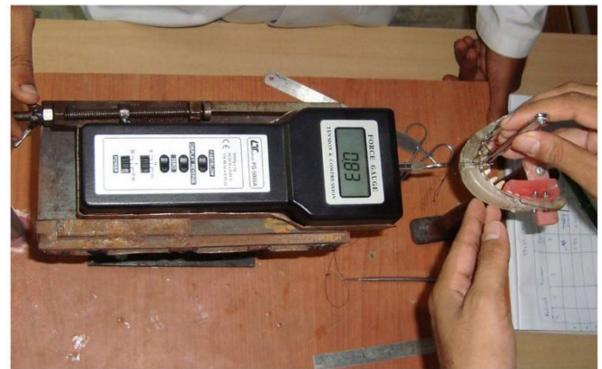
Fig 13: Force gauge showing reading for root displacement measured with the divider
