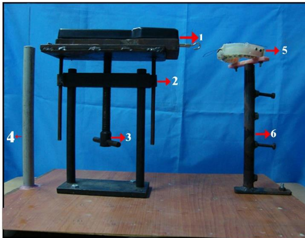
Fig 10: Alignment of the force measuring gauge with the tyodont assembly
