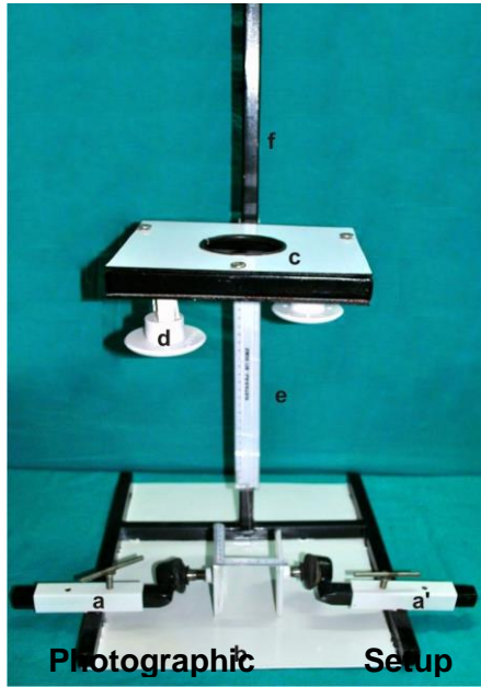
Standardized photographic set-up (FIGURE 2)
