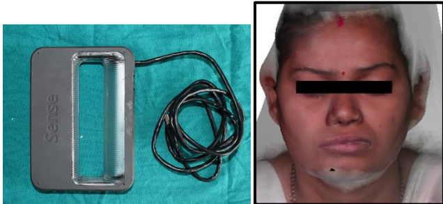
Figure 3 Structured light based scanner. Figure 4 3D scan
