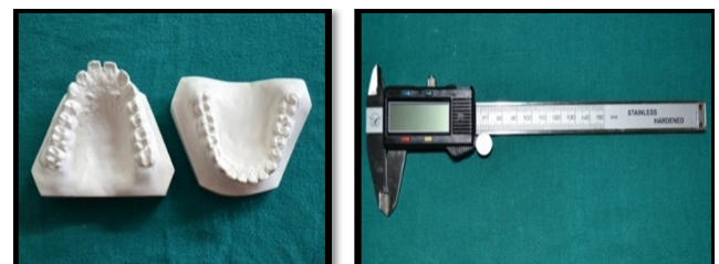
Figure 2: Digital caliper used for taking dental casts measurements
