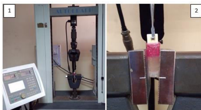
Figure 2: Universal testing machine for testing the shear- bond strength (1) and the schematic illustration showing the specimen being tested on the machine (2)
