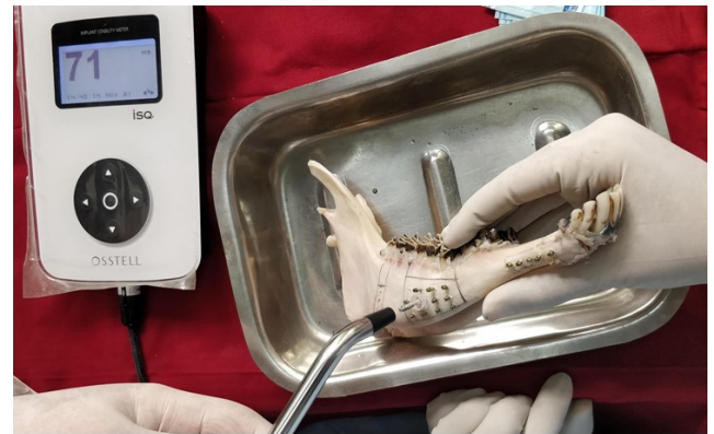
Figure 8: Primary stability of each implant measured using Osstell ISQ on Jaw 1
