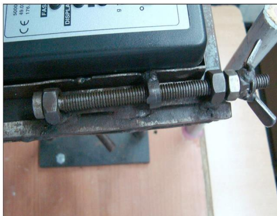
Fig 11. Bolt guided by the nuts to move the force gauge forward (or) backward
